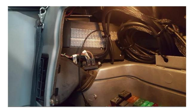
4. **2007 T600**: Mounted behind the gauge cluster secured with tie wraps to the large wiring harness.
