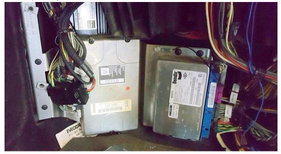
4. **2007 T2000**: The J1708 connection points are behind the dash, to the left of the glove box. Refer to the ER-SV2 HDV Guide for J1708 testing information.
