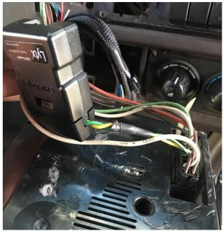
6. **2012-2016 T880**: The J1939 backbone can be found left of the gauge cluster, right above the ignition key.
